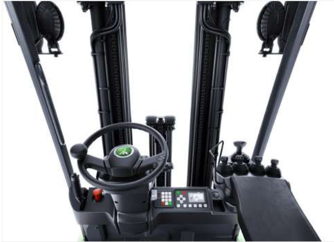
Excellent visibility through the mast with low dashboard including built-in display with essential driver information and functions.
